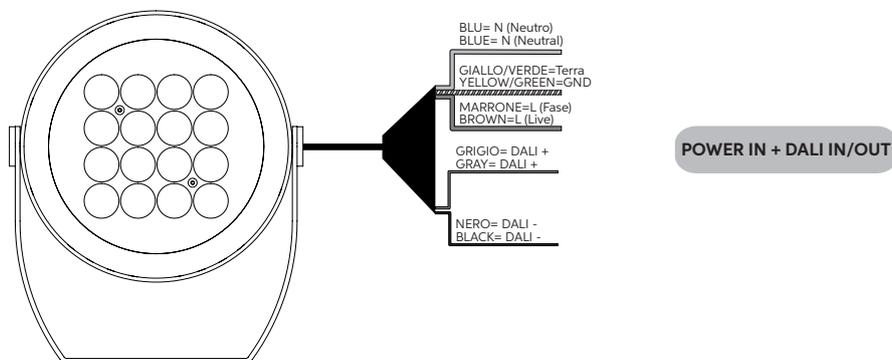
Note: the power and DATA connection can be carried out by using the optional connection kit. Follow the instructions provided along with the connection kit.
