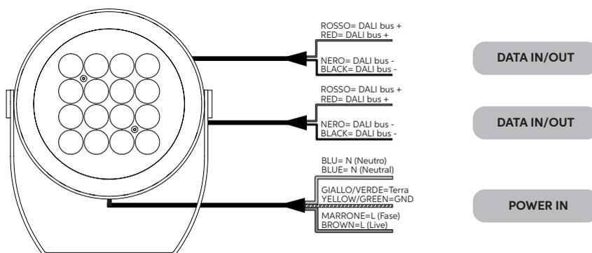
**“M” type cable ( hybrid cable for DALI without connectors )**
